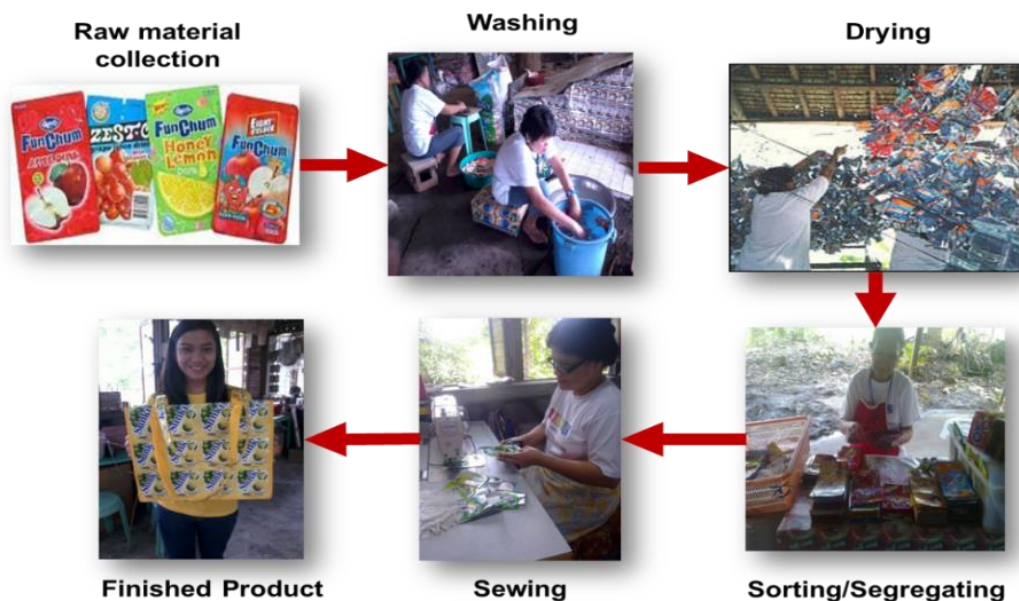
Fig. 2. Steps in producing bags out of used tetra packs
