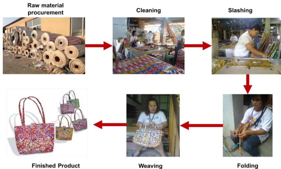
Fig. 3. Steps in producing bags out of rejected tetra pack material
