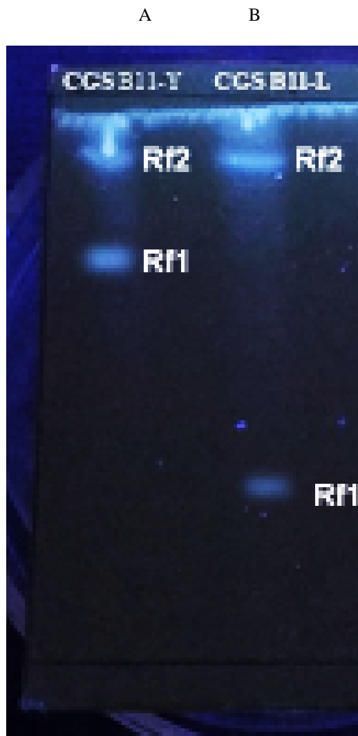
Fig. 3. Thin layer chromatography profile of Lanthanum-treated Streptomyces angustmyceticus strain CGS B11. Lane A: R_f1= 0.73 , R_f2= 0.90 ; Lane B: R_f1= 0.33 , R_f2= 0.90 .
